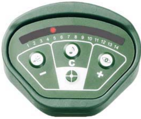
Figure 2: Visual alarm indication on the left side of the bar graph of an aluminium object, 16 mm diameter and 50 mm long.
