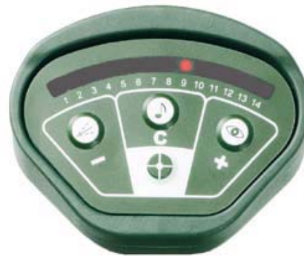
FIGURE 1 Visual alarm indication on the right side of the bar graph of a ferrous object, a BLU-26
