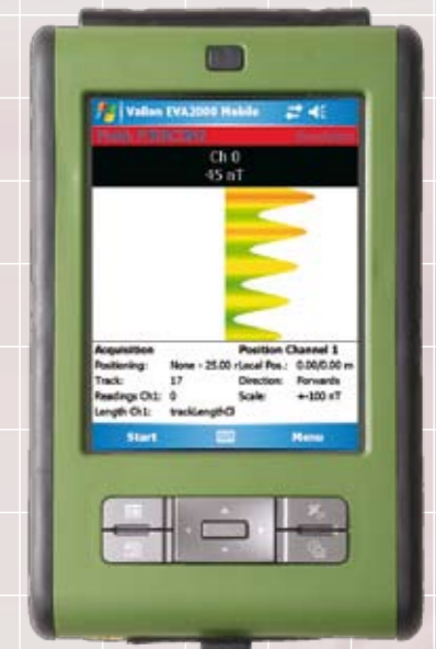
Real-time data monitoring: scrolling curve of survey data
