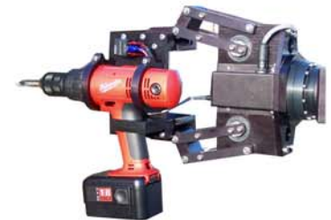
Drill Milwaukee 18V battery. Electrically disconnects when released.
